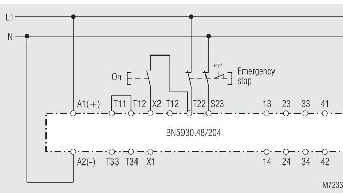
Two-channel emergency stop circuit with "Cross fault detection" in the alternating current network.
