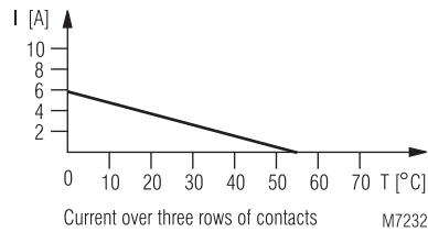
Continuous current limit curves depend on the ambient temperature
