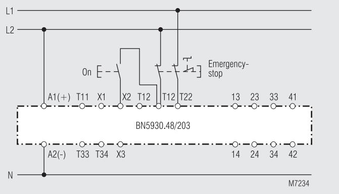
Two-channel emergency stop circuit. "Emergency stop" connected at two different phases, thereby giving "Cross fault detection".
